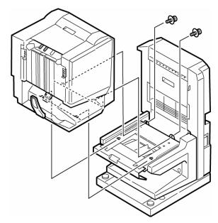
10. Lift the locking piece back up and tighten the screw firmly. Be sure it's out of the way and the screw is tight—otherwise the platform will not move freely.
